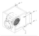
**Installation of the appliance:** after deciding the position and the type of installation, insert the anti-vibration rubber caps in the holes of the brackets supplied fig. 5C.
