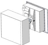
then insert the supply cord in the plastic pipe. Fix the appliance without the stain-less steel external body, which was previously removed from the motor block, by matching the holes of the motor block with the holes on the wall. Tighten with the screws supplied.
