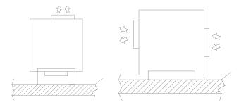
Note: in the vertical fixing, the brackets supplied can be used only on the longest side fig. 4.
