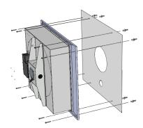
(fig. 2) drill all the holes marked on it into the external wall, by paying attention not to damage water pipes or power lines. The holes on the wall are to be drilled with a 8 mm. bit.
