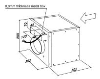
The appliance is designed to exhaust fumes and odours very silently and in the best way. It must be installed in the house and connected to the cooker-hood, which is in the kitchen fig.1.
